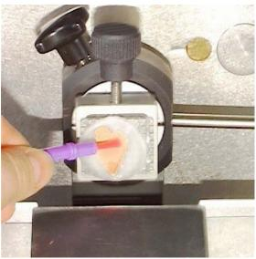
Figure 29. Coating the block with Oil.
