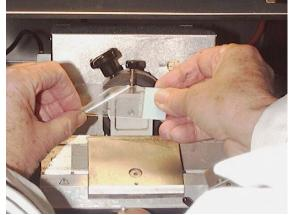
*Figure 7. Peeling mylar from adhesive coated slide.*
