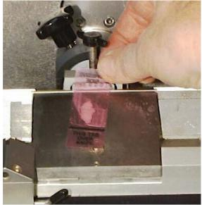
Figure 13. Handling the cut section.
