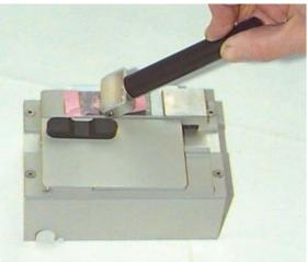
Figure 15. Laminating the section to the Slide.
