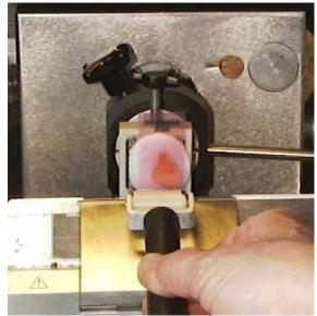
Figure 11. Laminating the Tape to the block face.
