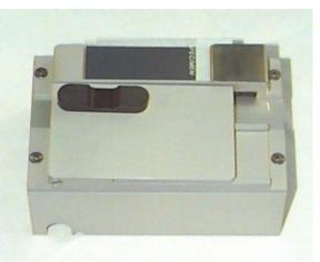
*Figure 8.* Adhesive Coated Slide on Blue/Gray Pad.
