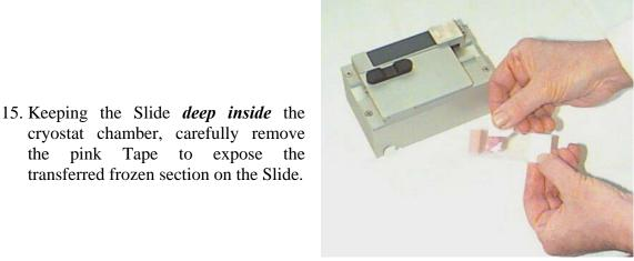
Figure 19. Removing Tape from cured Slide.
