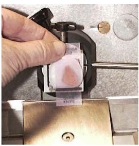
Figure 10. Placing Tape on block face.
