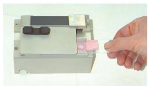
Figure 16. Placing the slide into the Flash Tray.
