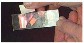
Figure 20. Technique for removing Tape from Slide.
